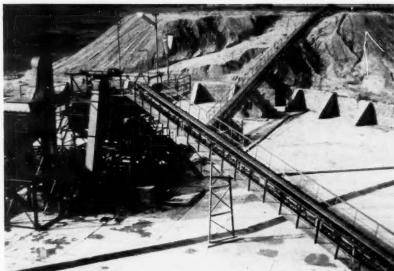
KIMBERLITE washing plant at Bakwanga, Congo Republic. The undisintegrated ore from plant washing is conveyed to piles at right for weathering before treatment.
